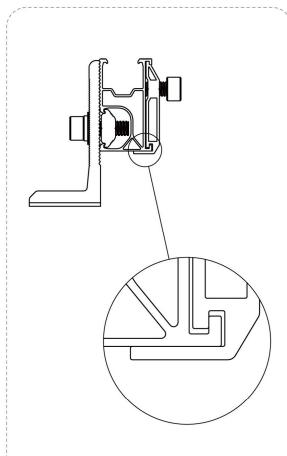
the additional bottom supporting to two joining rails provides additional safety and strength and significantly increase the rail compressive capacity.
